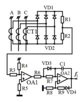
Fig. 5. Schematic diagram of the block calculating the emergency current of the stator of a synchronous generator.
