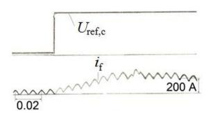
Fig. 9. Oscillogram of the increase in current in the excitation circuit during an abrupt action.
