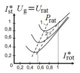
**Fig. 4.** Compounding characteristics of a synchronous generator.
