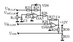
Fig. 7. Schematic diagram of the current compounding unit.
