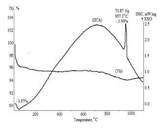
**Fig.3.** Thermal analysis results for DTA (1), TG (2) of the silica fume + NaCl composition
