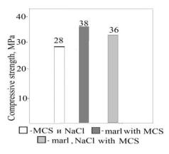
**Fig. 2**. Dependence of the strength of the material on the composition of the composition
