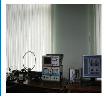
The developed now hardware-software system provides for the registration of a large number of PD pulses and their cumulative amplitude distribution. Determined by this characteristic, parameters are the following: the average apparent charge, the maximum apparent charge, the pulse repetition rate and an average current of PD. Analysis of a variety of experimental data has shown that the most effective representation of the data are the PD signals gain-phase diagrams (GPD).
