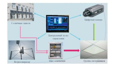
Fig. 3. Block diagram of the demonstration and laboratory complex of the intelligent artificial lighting systems and alternative energy
