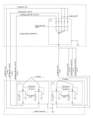
Fig .6. Diagram of 10 kV cable lines polygon
