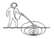
Fig .3. Induced signals in the induction method.
