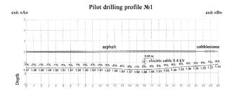
$Fig. 8. \qquad Pilot \ drilling \ profile \ of \ cross-linked \ polyethylene \ insulated \ cable$
