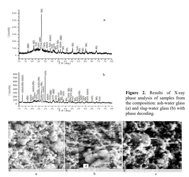
**Figure 3.** Microstructure of fractures of samples of compositions of compositions: ash with water glass (a, b, d), slag with water glass (c), fired in a muffle (a) and microwave field (b-d).
