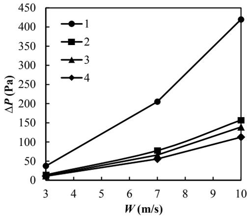
FIGURE 6. Relationship curves between pressure drop and gas inlet velocity for various slot height  $h_{sl}$ , mm: 1 – 15; 2 – 30; 3 – 45; 4 – 60 (at inlet gas velocity  $W = 10$  m/s).
