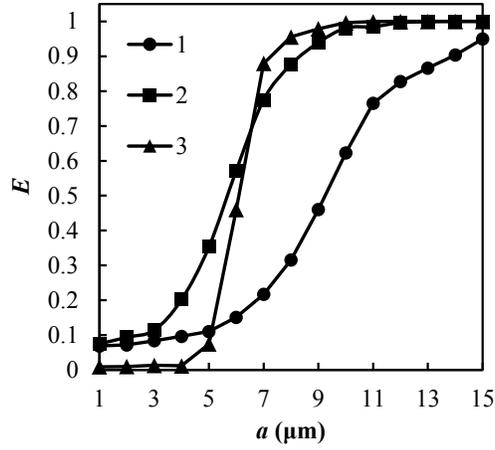
FIGURE 4. Separation efficiency versus particle diameter for various gas inlet velocity  $W$ , m/s: 1 – 3; 2 – 7; 3 – 10 (at slot height  $h_{sl} = 30$  mm).
