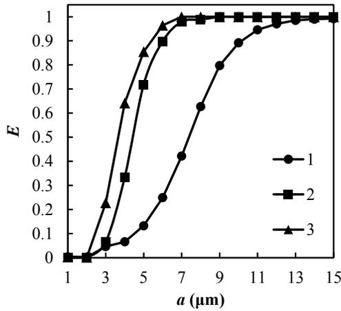
FIGURE 5. Separation efficiency versus particle diameter for various gas inlet velocity  $W$ , m/s: 1 – 3; 2 – 7; 3 – 10 (at slot height  $h_{sl} = 45$  mm).
