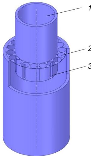
**FIGURE 1.** 3D model of the multivortex separator with coaxial tubes: 1 – gas inlet; 2 – plate with outlet holes for purified gas; 3 – rectangular slots.
