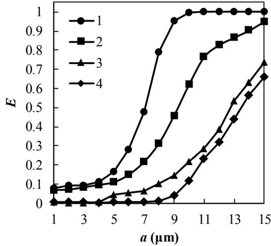
**FIGURE 2.** Separation efficiency versus particle diameter for various slot height  $h_{sl}$ , mm: 1 – 15; 2 – 30; 3 – 45; 4 – 60 (at inlet gas velocity  $W = 3$  m/s).
