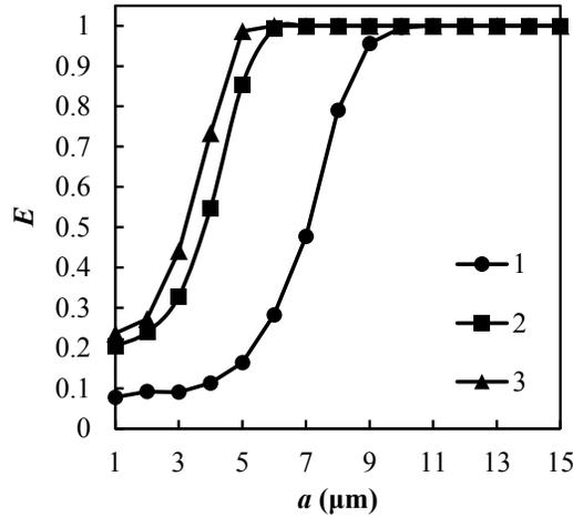
**FIGURE 3.** Separation efficiency versus particle diameter for various gas inlet velocity  $W$ , m/s: 1 – 3; 2 – 7; 3 – 10 (at slot height  $h_{sl} = 15$  mm).
